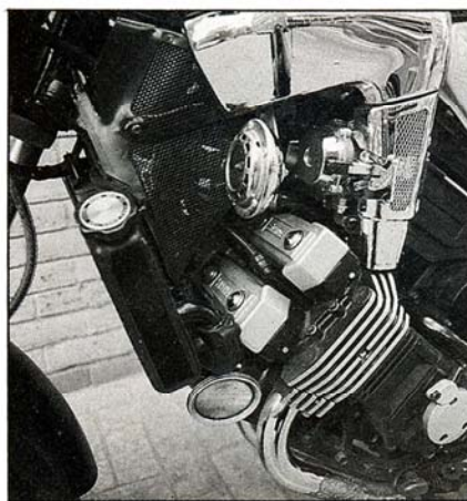
Dummy air scoops, fin edges and chrome pipes trace air flow through Yam motor
