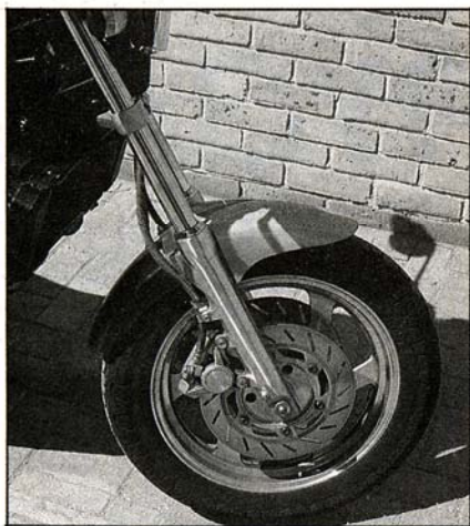
16-inch wheel means Yam steers quickly, opposed-piston brakes are superb
